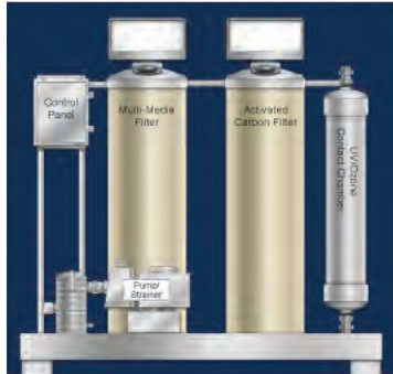
RECLAIM SYSTEM (SKID)
